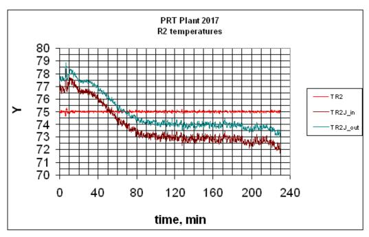
Very constant reaction temperature in R2. Decreasing cooling shows increasing polymerization rate.
