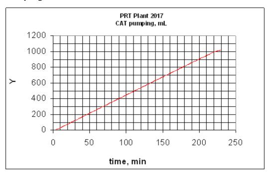
Catalyst slurry feed is constant. Starting with 1500mL filling, catalyst is consumed after 220min at CAT=60
