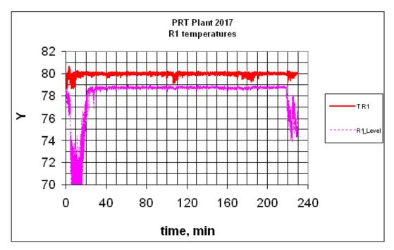
The temperature difference between TR1 and "level temperature" indicates the slurry level in R1.
