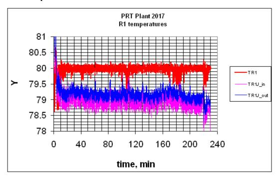
Very constant reaction temperature TR1. Temperature difference between reactor content TR1 and cooling water temperature TR1J\_in and TR1J\_out represents polymerization rate.
