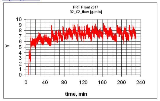
The overall C2 feed to R2 contains currently the amount of C2 that is required for purging the H2 concentration down (to 4.5%, see above). Near to steady state the value was 450g/h.
