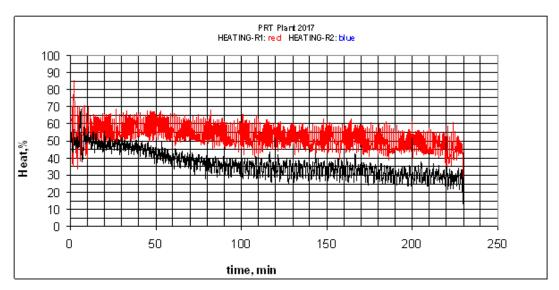
Decreasing heating capacity indicates increasing polymerization heat.
