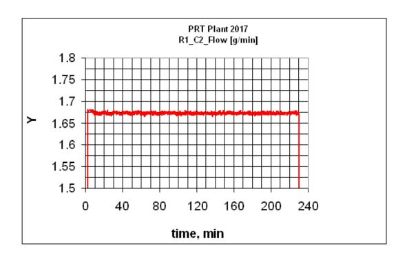
C2 feed to R1 was set constant at 1.675g/min = 100.5g/h. This - together with the overall C6 feed to R1 (C6 feed + catalyst feed) - determines the R1 solid content. The final solid content in steady state can be "designed" at the beginning of the experiment.
