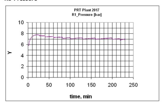
The chosen process control mode allows quick finding of steady state. Sampling causes quick pressure decrease: 9 samples have been taken.
